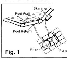
blocks and position it so the valve handle is facing away from the pool. Place the pump to the right of the filter as shown in Fig. 1.
