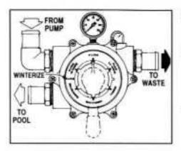
BACKWASH: Backwashing reverses the flow of water through the filter to flush out the dirt and debris, and waste water is discharged to waste from the valve body port with sight plass.
