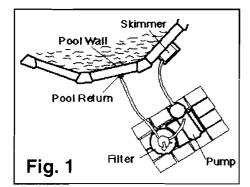
Place the pump to the right of the filter as shown in Fig. 1.
